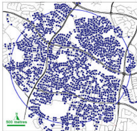
(C) Using the captured streets, the program generates a list of all possible addresses and sends this list to the geocoding engine of the GIS, creating points at all possible addresses.
