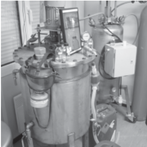
Pressure reaction vessel in the foreground and background – utilising PMK in MDMA production. Synthetic Drugs Unit, Helmond, Holland 2004.
