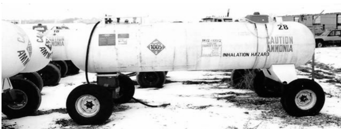
Anhydrous Ammonia Tanks: Source Cain (2004a).
